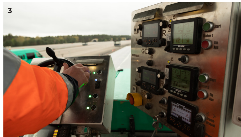
1 Production lane to lane - patented control technology via scanning | 2 Grinding/grooving shaft - variable composition for optimised surface design | 3 modern measuring and control technology - increase in process/product quality
