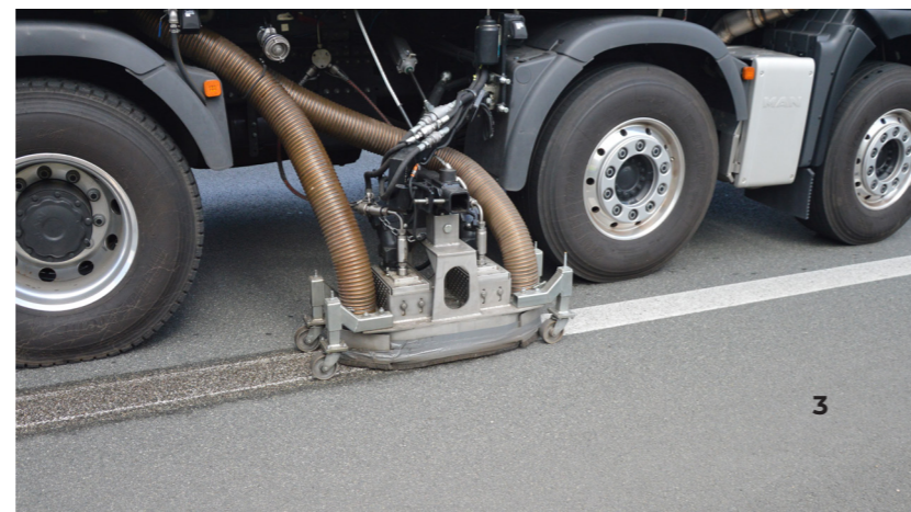
1 Computer control in the cab | 2 use of the rear cleaner | 3 use of the side cleaner
